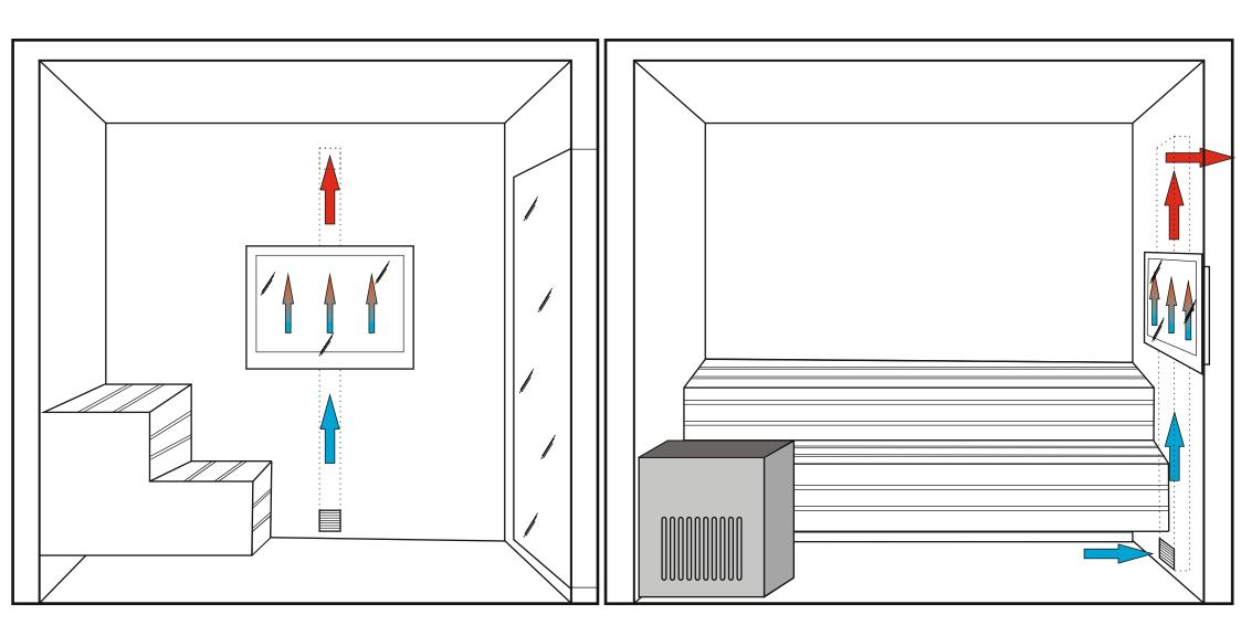
The ventilation duct shall deliver cool air to the middle-bottom part of the TV mounting box, and exhaust the heated up air from the middle of the top part. The ventilation duct cross-section is to be equivalent to at least 100 mm diameter tube.
