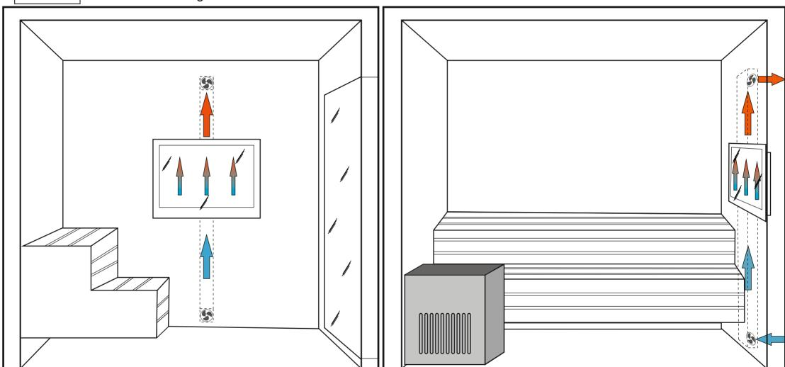
The ventilation duct must have forced ventilation and supply cold air from outside the room to the lower part of the TV installation box, centrally, while removing the heated air from the upper part.
